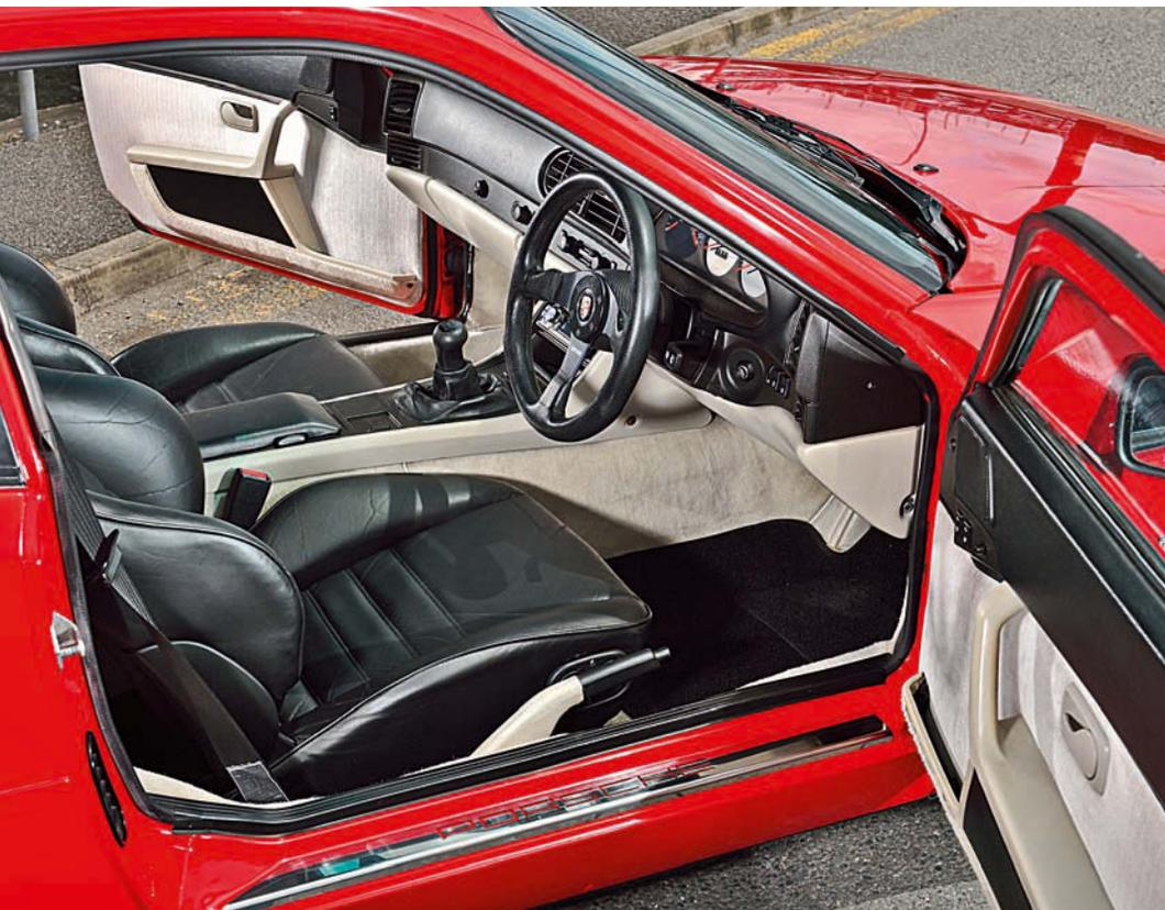
Inside refurbished 944 Turbo seats are joined by a Momo steering wheel and a short-shift kit to improve the car's touch points...
